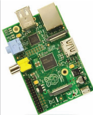
The Raspberry Pi Model A board uses the same 700-MHz ARM1176 Broadcom BCM2835 processor as the Model B board but includes as standard only 256 MBytes of RAM.
