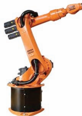
Figure 3 In this serial robot, a series of links is connected by motor-actuated joints that extend from a base to an end effector.
