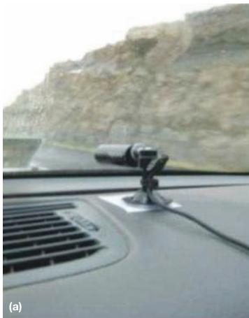
The typical dashboard camera uses a suction mount to connect it to the front window (a). Some models, however, have a distracting screen that is in the driver’s line of sight (b).
